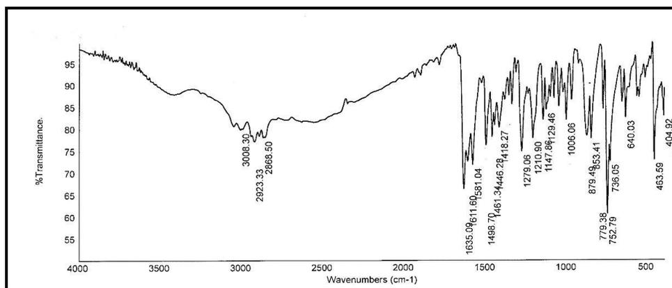
Fig (1) IR spectrum of the Schiff base [I]
