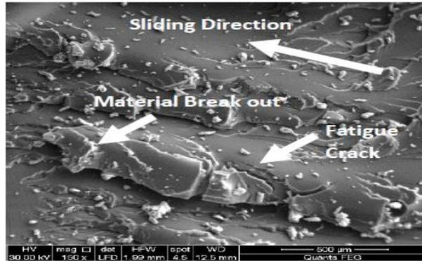
**Fig (5)** SEM micrograph of worn surface for the neat epoxy specimen after dry sliding against a stainless-steel disc under a load of 90 N and sliding velocity of 3 m/s for 900 sec.
