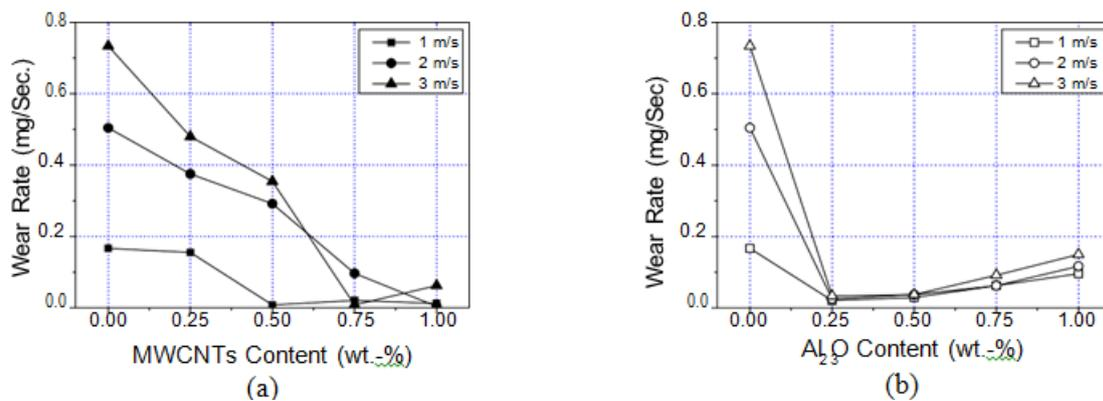
Fig (3) Variation of the wear rate with weight percent of MWCNTs (a) and Al<sub>2</sub>O<sub>3</sub> nanoparticles (b) at constant load of 90 N and several sliding velocities.
