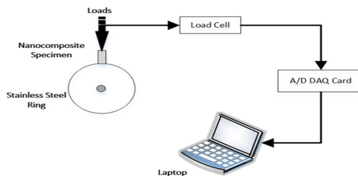
Fig (1) Aschematic illustration of the pin-on-ring wear tester
