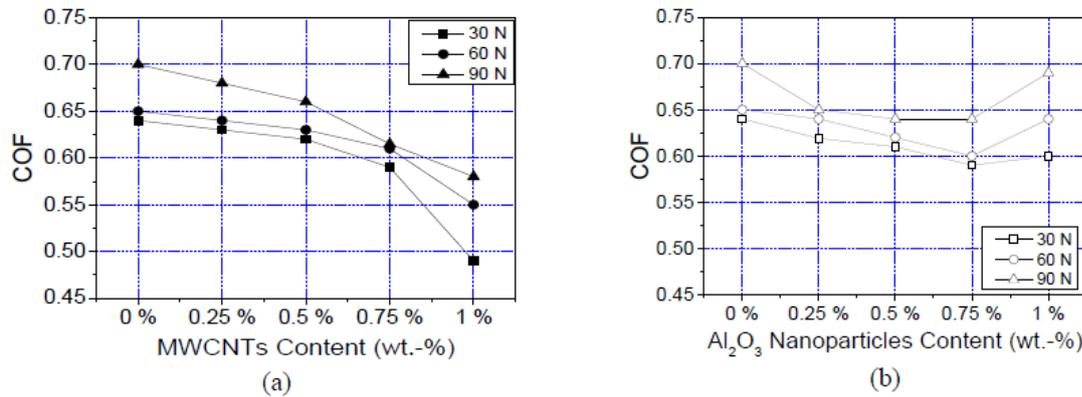
Fig (2) Variation of the cof with weight percent of mwcnts (a) and al<sub>2</sub>o<sub>3</sub> nanoparticles (b) at constant sliding velocity of 3 m/s and different loads.
